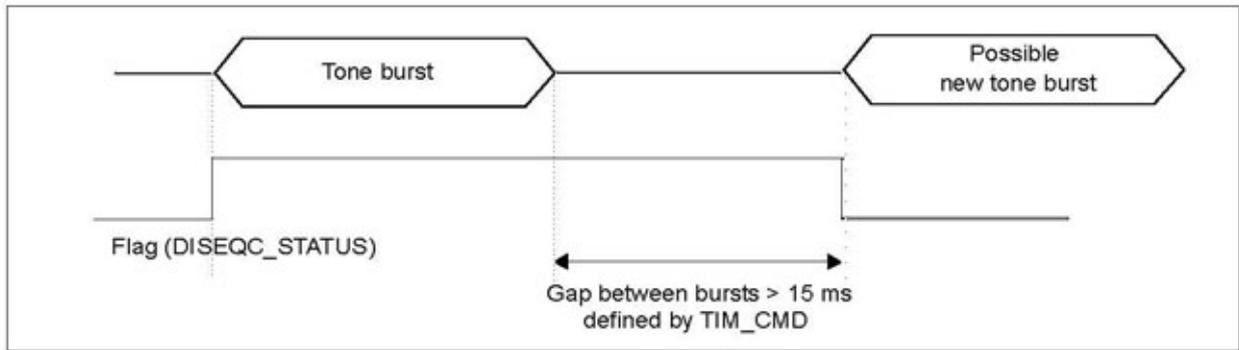
The backward compatibility of DiSEqC requires a 15-ms gap after a tone burst sequence. This information is delivered by a flag in a status register. This flag is set at the beginning of the transmission, and is reset after a time which includes both the transmission and a period defined by the I2C bus.
