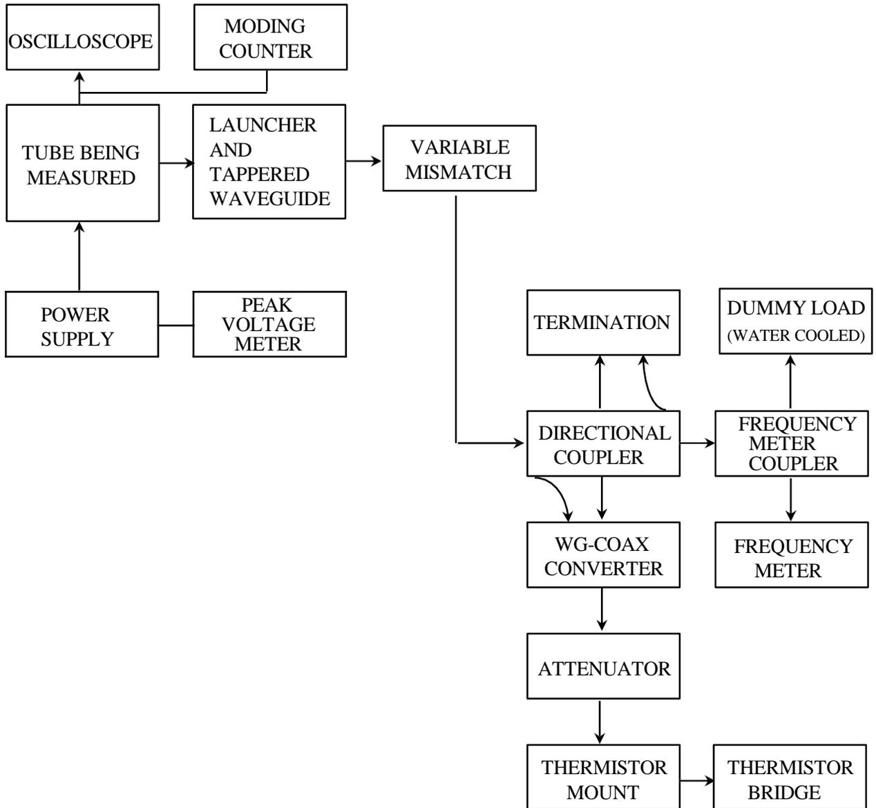
**LAUNCHER AND TAPERED WAVEGUIDE FOR TESTING**
