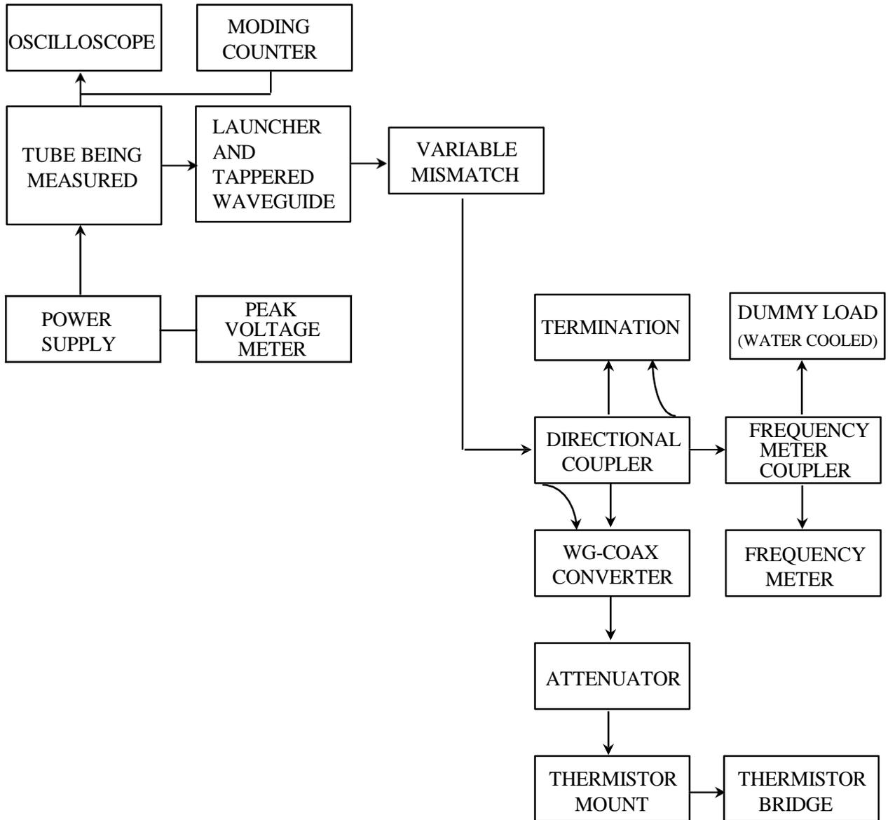
**LAUNCHER AND TAPERED WAVEGUIDE FOR TESTING**
